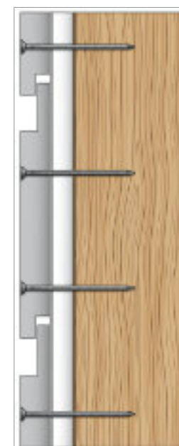
All nails should be countersunk and filled over
